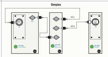
With an additional loss meter and a 1x2 optical switch, hybrid simplex assemblies can be efficiently tested. The two master test jumpers and detectors are configured for the different connectors of the hybrid assembly.
